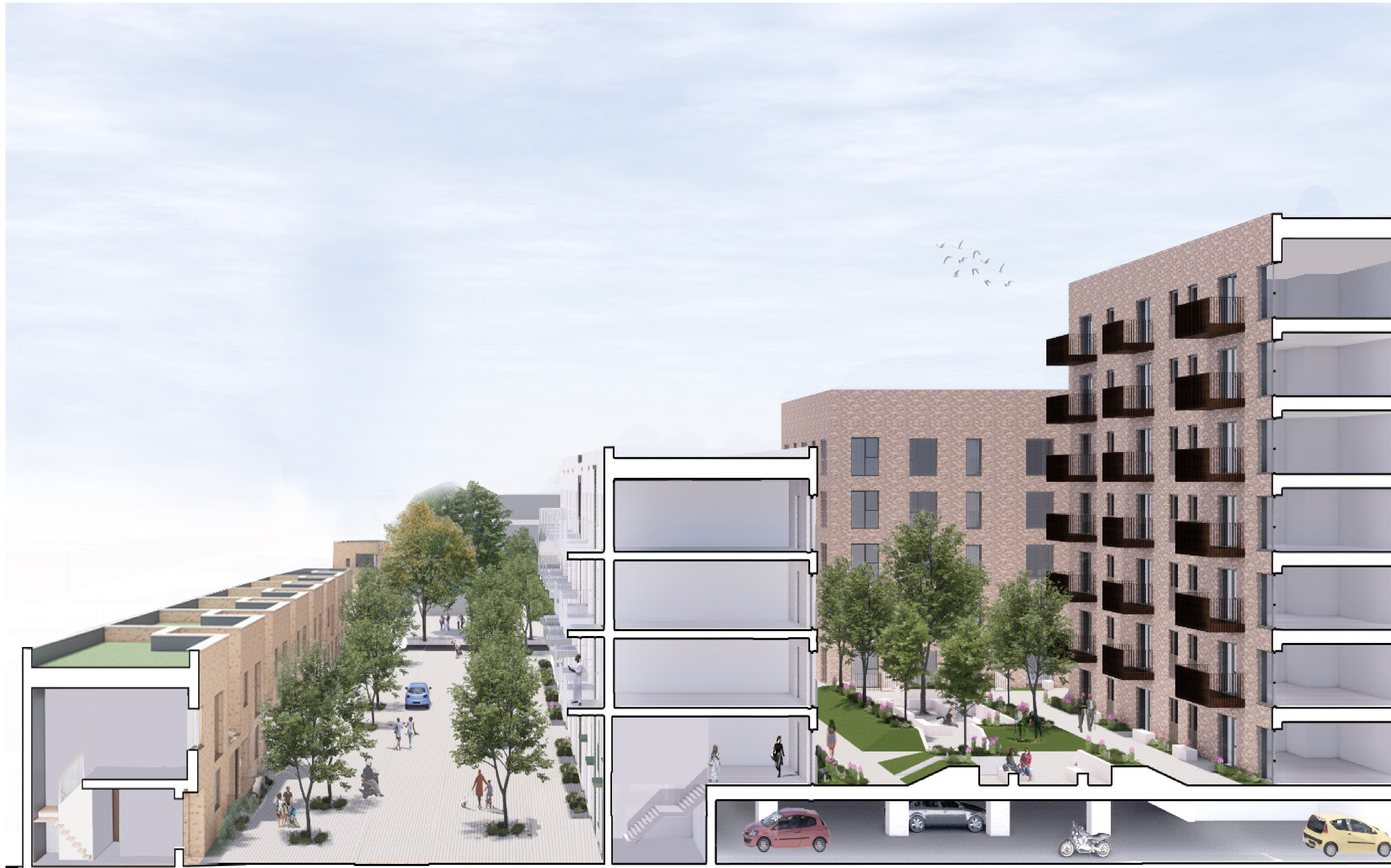
A cut through sketch showing the first floor resident only courtyard with parking below
